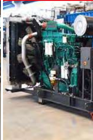
800 KVA BF WITH DUAL BATTERY SYSTEM
